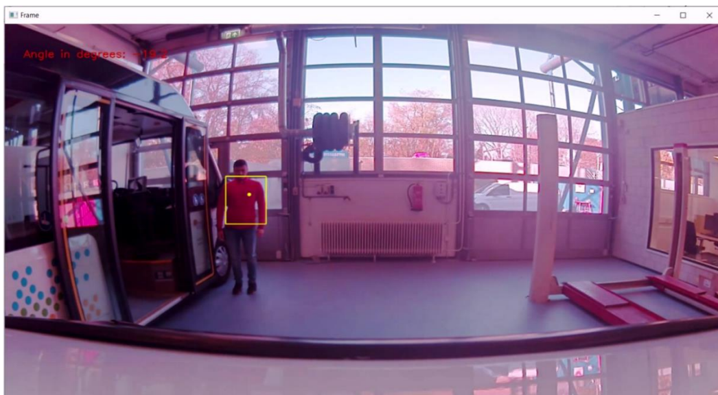
Figure 17: Figure showing angle to person is -19.2 degrees.
