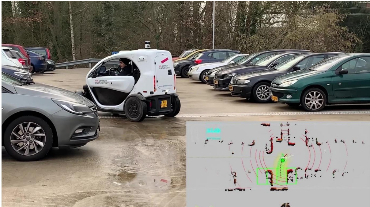
Figure 14: Vehicle parking into one of the defined parking spots.
