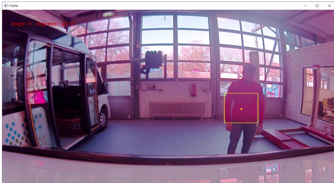
Figure 18: Figure showing angle to person is 26 degrees.
