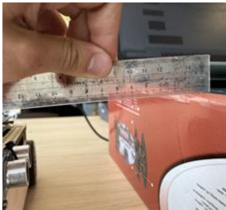
Figure 4. Comparing the distance between the ultrasonic sensor and the box to the real distance
